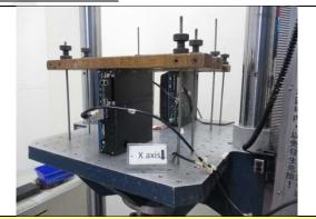
Mechanical Shock Test (-X axis)
