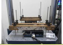
10. Mechanical Shock Test (+Z axis)
