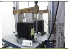
Mechanical Shock Test (+Y axis)
